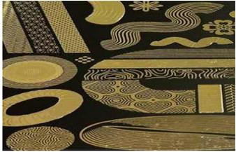
This Image shows foil on foil .We can also enhance this with polymer on top ,sealing and enhancing the spot image
