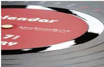
Standard spot varnish is showcased here with exceptional accuracy .We register accurately with 4 cameras making in line adjustments.
